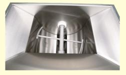
PADDLE SHOWN INSTALLED IN HOPPER
